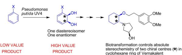
Figure 1 Reaction scheme for the formation of *cis*-dihydrodiols from monosubstituted aromatics leading to the formation of Vernakalant
